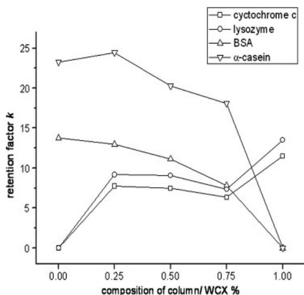
**Figure 3.** Effect of column composition on retention factor. The conditions were the same as in Fig. 2C.
