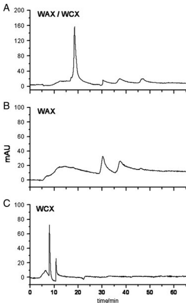
**Figure 5.** Separation of proteins extracted from rat liver with the mixed-bed (WAX/WCX = 1:1, w/w) ion-exchange column (A), WAX column (B) and WCX column (C). The ion-exchange columns were of the same size of 0.3 mm id  $\times$  100 mm. Mobile phase A: 10 mM Tris-HCl (pH 8.3)+10% ACN; B: A+2 M NaCl (pH 8.3)+10% ACN. Gradient profile: 0–15 min. 0% B, 15–25 min 10% B, 25–35 min 30% B, 35–45 min 50% B, 45–55 min 80% B and 55–65 min 100% B. Injection, 10  $\mu$ g.
