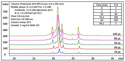
Proteomix<sup>®</sup> SCX vs. Antibodix<sup>™</sup> WCX using a salt and pH gradient for the analysis of MAb 321
