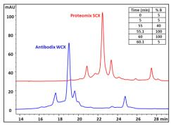
Mobile phase: A: 2.4 mM Tris, 1.5 mM Imidazole, 11.6 mM piperazine pH 6 and B: A + 0.5 M NaCl pH 10.5; Flow rate: 0.8 mL/min; Column temperature:  $30^{\circ}$ C; Sample: 10 µL MAb 321 (5 mg/mL)
